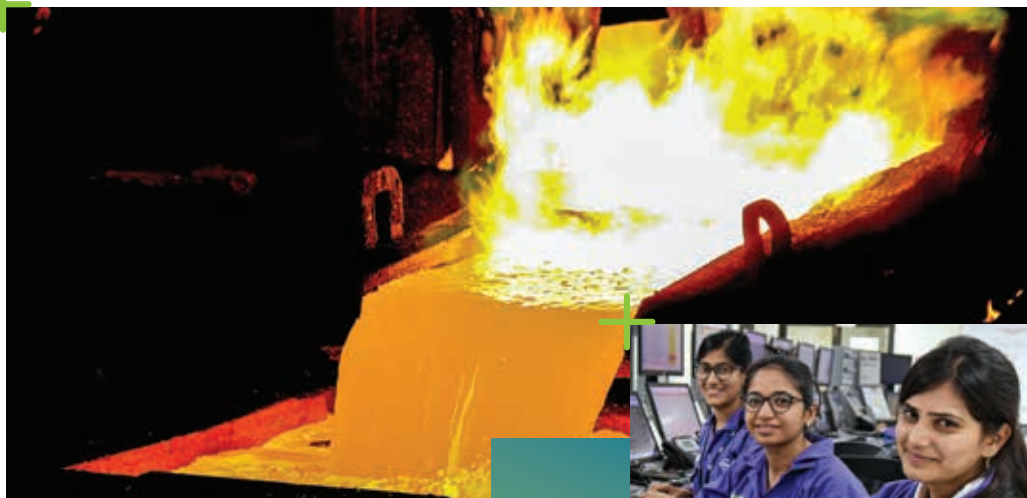
Above: Molten copper pouring from the launders
