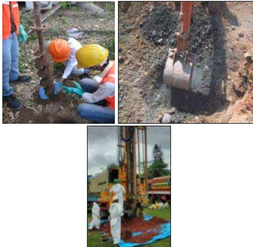
**Figure A.2.2 Examples of Soil Sampling Methods**
