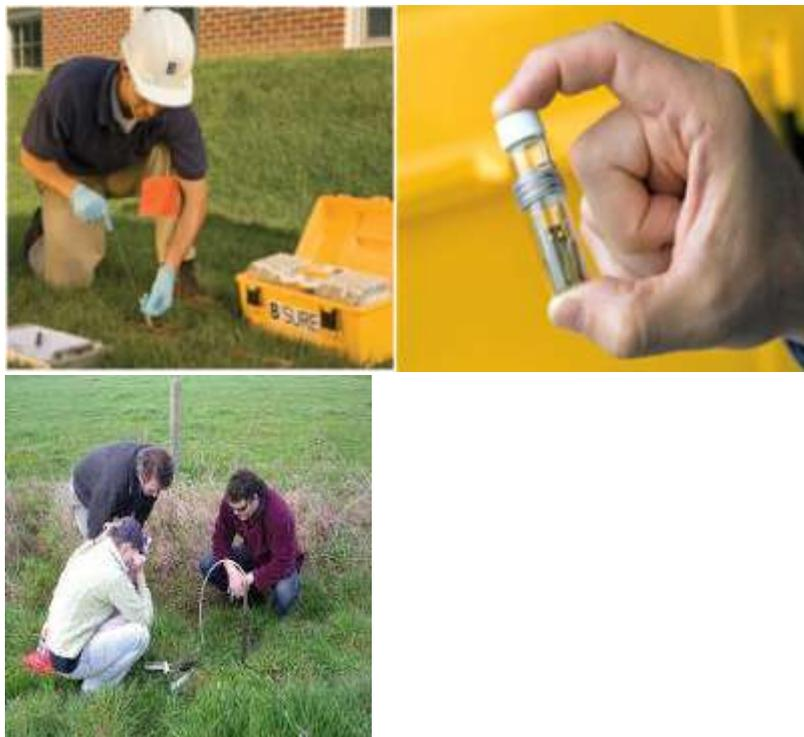
**Figure A.2.3 Examples of Soil Gas Sampling Methods**
